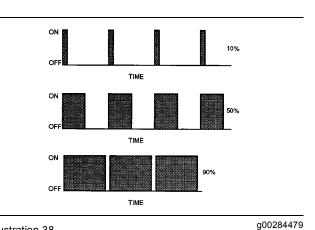
Illustration 38 Example Of Pulse Width Modulation
