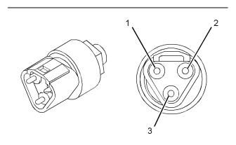
Illustration 28 Engine oil pressure sensor g01133306
