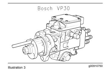
The Bosch VP30 fuel injection pump is installed on the engine. The fuel injection pump conforms to current emissions. Both the pump timing and the high idle are preset at the factory. The fuel injection pump is not serviceable. Adjustments to the fuel injection pump timing and high idle should only be made by personnel which have had the correct training. The fuel injection pump uses the engine ECM to control the engine RPM.
