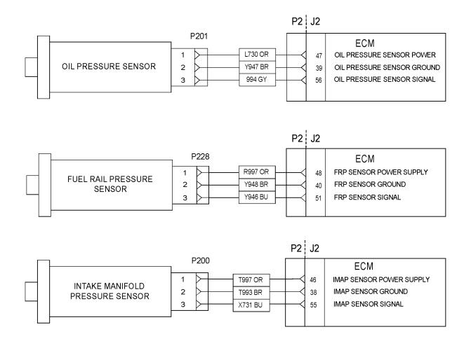
Illustration 35 Schematic for pressure sensors
