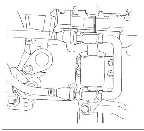
Illustration 23 Electric fuel priming pump g01201623
