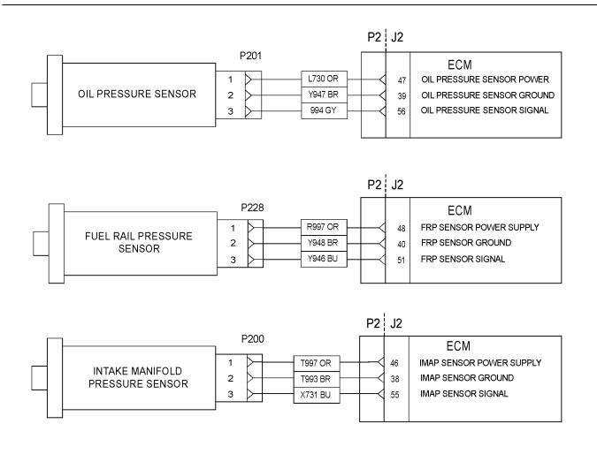
Illustration 38 Schematic for pressure sensors
