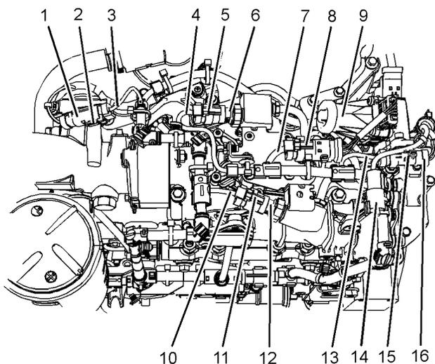
1. If the Diesel Particulate Filter (DPF) assembly is mounted on the valve mechanism cover, removal of the DPF assembly will be necessary in order to access the NRS induction mixer. Refer to Disassembly and Assembly, "Diesel Particulate Filter - Remove" for the correct procedure.
