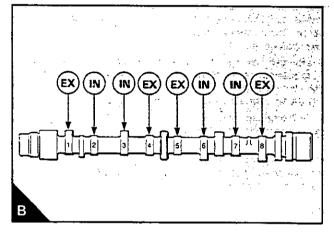
7 Remove the camshaft clamps and remove the camshaft (12A.07/A). Remove the seals from the camshaft.
