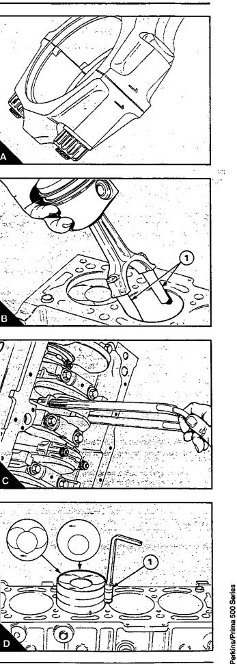
6 Push the piston and connecting rod assembly through the bore and onto the crank pin. If piston cooling jets are fitted, the assembly must be turned to ensure that the connecting rod will not hit the jet as the rod is fitted. When the connecting rod has passed the piston cooling jet, turn the connecting rod until the arrow on the top of the piston is towards the front of the engine.
