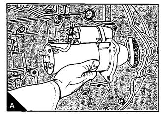
I For M80R starter motors, the brush assembly and the armature assembly can be fitted into the body together but they will be pulled into position by the effect of the magnets. Ensure that the thrust washer remains in position on the front of the armature shaft.
