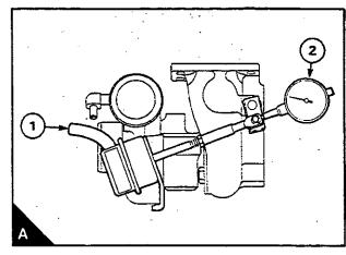
2 Check that the pressure needed to move the rod 0,38 mm
