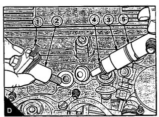
I is tight in the cylinder head, use the slide hammer (A1) and the I relevant adaptor (A2).
