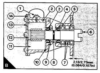
4 Support the pump on the cover end and press the shaft and bearing assembly into the bearing housing. When the assembly has been correctly pressed in, the outside bearing will have a protrusion of 2,13/2,73 mm (0.084/0.107 in) from the mounting face.
